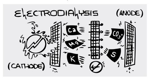
As the ions are separated by this process, they wind up in **separate compartments**. Each compartment has its own water outlet, and each compartment is releasing water when your ionizer is making ionized water.
